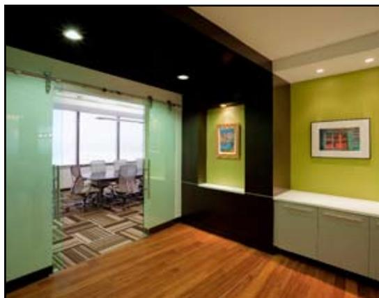
Energy saving techniques like reconfiguring the work space to an open office design and positioning closed offices along interior walls, allowed the firm to maximize natural lighting throughout. This provided every employee natural light and minimized the need for interior lighting fixtures, which saved on upfront cost and will conserve energy in the future.
