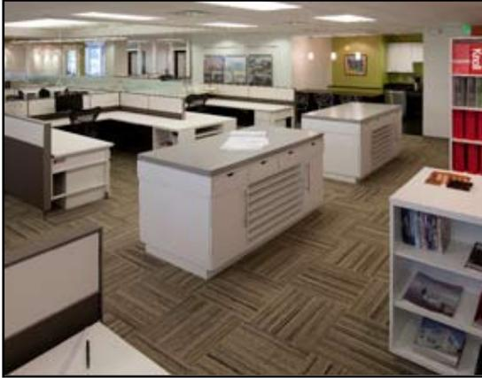
Materials designed and specified on this project for LEED certified qualification were, Teragren Bamboo Wood Flooring, Armstrong natural linoleum, and InterfaceFLOR which is comprised of 35% pre-consumer recycled content and 33% post-consumer recycled content. All cabinetry was produced from green board. No urea formaldehyde was added during the manufacturing process of the cabinetry. It was finished with low VOC paints.
